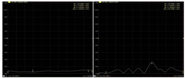
Figure left: Input VSWR S11 ( Pin=-30dBm, Load VSWR≤1.2, 25°C ), for reference only. Figure right: Output VSWR S22 ( Pin=-30dBm, Load VSWR≤1.2, 25°C), for reference only.
