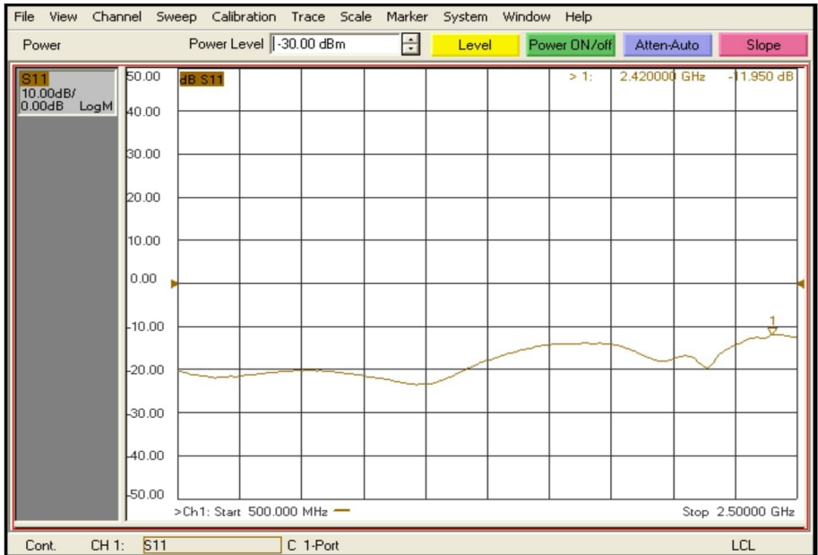
Input Return loss S11 (Pin=-30dBm, CW, Load VSWR≤1.2, 25°C), for reference only
