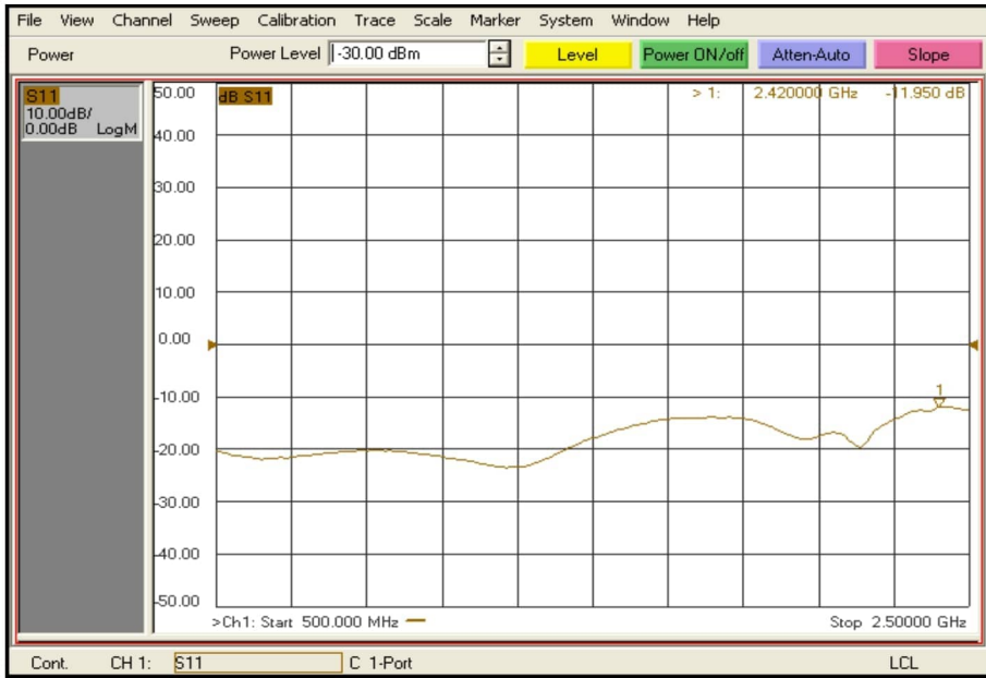
Input Return loss S11 (Pin=-30dBm, CW, Load VSWR≤1.2, 25°C), for reference only
